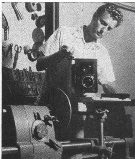
THE GOWLAND FLEX , a 4x5-inch twin lens reflex camera Pete designed (above) was built in home shop. The camera simplifies picture-taking by cutting out eleven operations, will be on the market this year.
